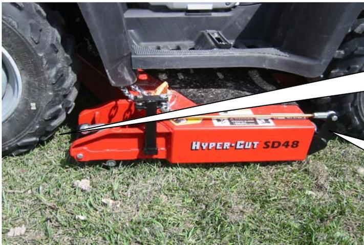
Check for clearance at the front wheels at upper and lower height extremes of steering movement!
