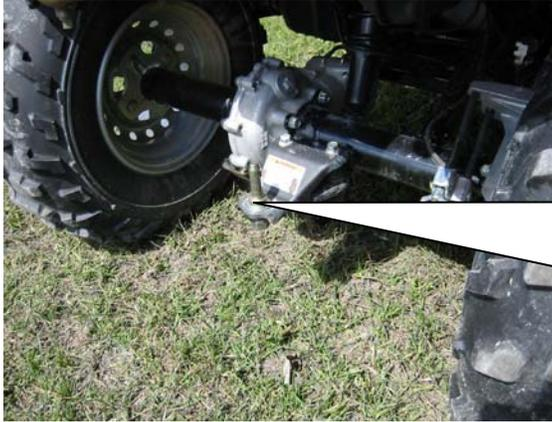
**NOTE** – tighten the hitch pin securely – to 150 ft-lbs (230.5 Nm). The HyperCut is “pushed” by the ATV through the hitch pin, this must be secure as instructed - failure to do so will result in damage to the ATV or the mower and/or both – or personal injury to the operator.
