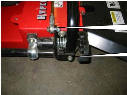
Remove this hardware in order to install the height control lever bolt.
