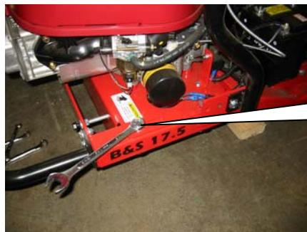
Vertical bolts (with wrench in place) are to lock the engine plate in place and the bolts at the rear are to provide tension.
