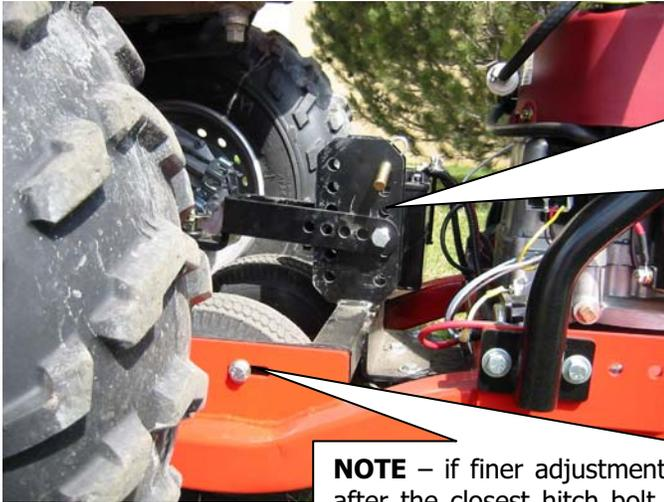
**NOTE** – the hitch with the swivel can be installed in either the “L – UP” or “L-Down” positions as shown. What is important is that the floating hitch member is in the horizontal position when installed on your ATV!
